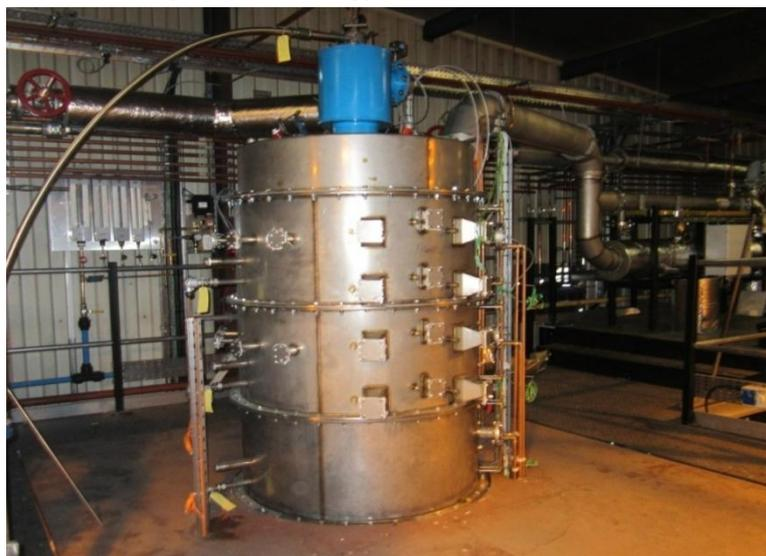
Figure 20: 250 kW vertically down fired oxy-fuel combustion chamber at PACT facilities, Sheffield.
